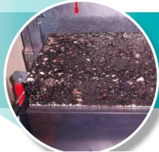
沥青混合料试件向上移动脱模 Asphalt sample moved upward for demoulding
