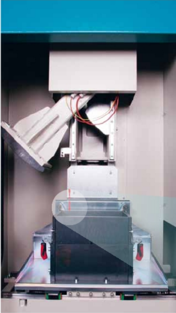
扇形轧轮处于待机位置 Roller Sector in waiting position
